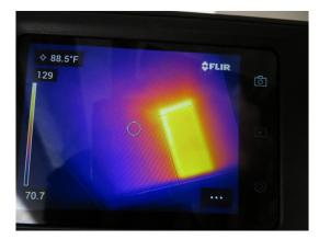
• There is evidence of possible previous water intrusion in one or more of the floors in the upstairs rear corner bedroom. Although all moisture content was within an acceptable level, this condition should be further evaluated and corrected as necessary.
